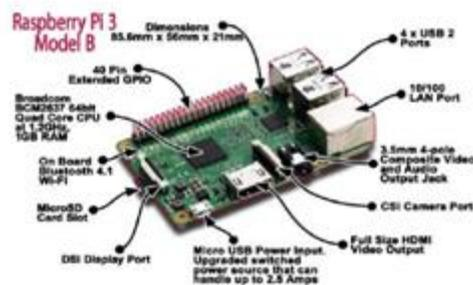
Fig.1 : Raspberry Pi 3 Model B
